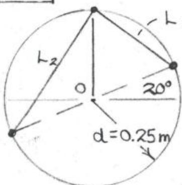
$$\begin{cases} L_1 = 2d \sin(90^\circ - 20^\circ)/2 = 0.287 \text{ m} \\ \delta_1 = 0.25\sqrt{2} - L_1 = 0.0668 \text{ m} \\ L_2 = 2d \sin(\frac{90^\circ + 20^\circ}{2}) = 0.410 \text{ m} \\ \delta_2 = L_2 - 0.25\sqrt{2} = 0.0560 \text{ m} \end{cases}$$
