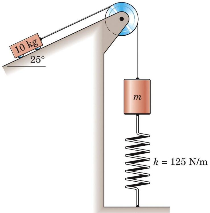
3/107 Let  $s$  be the slant distance down the incline traveled by the 10-kg cart.
